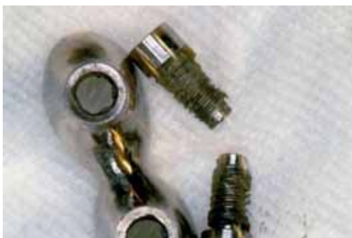
Fig. 1-1-2 Contamination around the screw that resulted from the loosening of the abutment screw
