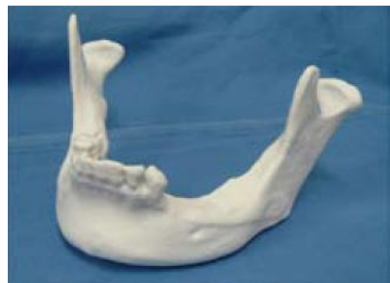
Fig.3-2-2 Three dimensional model. CAD data was formed from the DICOM data, then with the inkjet printer (Z403 3D printer® DICO) the additive manufacturing was conducted.
