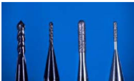
Fig. 4-1-40 Processing apparatus (Left to right) 2.0 mm, 1.0 mm super hard end-mills; 2.0 mm, 1.0 mm electroplated diamond burs
