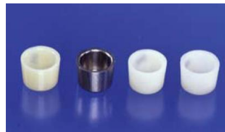
Fig. 4-1-41 Completed crown (Left) HR, Ti, CP, VP
