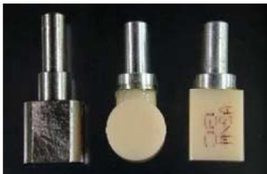
Fig. 4-1-57 Blocks of titanium, porcelain and resin used
