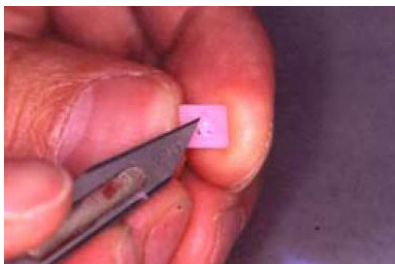
Fig. 4-2-37 Open a hole on the top of the pick-up coping with a design knife
