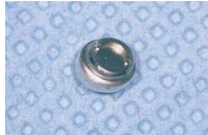
Fig. 4-3-14 Casting with the usual method for finish
