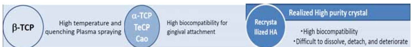
Fig. 4-2-2 Manufacturing process of recrystallized hydroxyapatite
